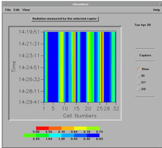
Figure 1: Application showing the beam loss distribution
