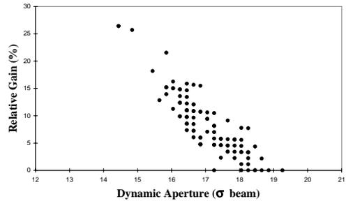
Figure 2: Relative gain as a function of the DA of the unsorted sequence of random errors for 100 realizations. All random errors.
