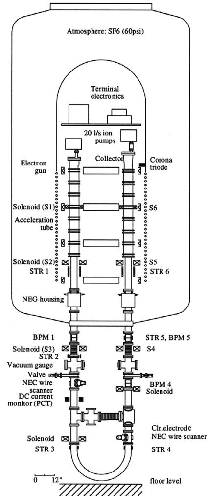
Figure 1: Recirculation system beamline layout.
