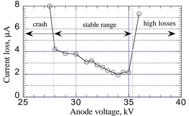
Figure 2: Measured dependence of losses on beam energy. Pelletron voltage was kept at 1.135 MV, beam current was 200 mA. Beam kinetic energy is  $eU_o + eU_A$ .
