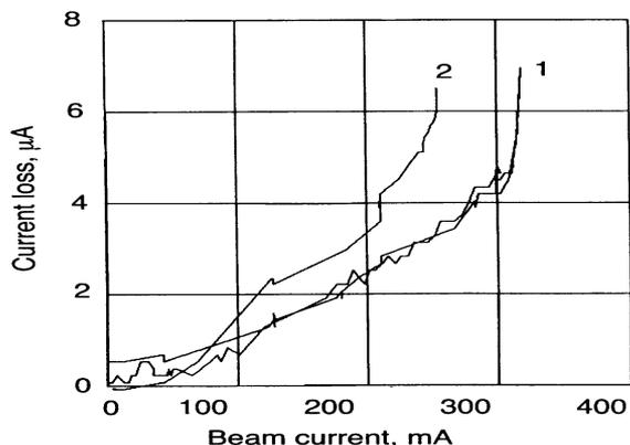
Figure 3: Measured current loss as a function of electron beam current. Curve (1) -  $p = 0.8-1.0 \cdot 10^{-7}$  Torr, (2) -  $2.3-3.3 \cdot 10^{-7}$  Torr.  $U_o = 1.135$  MV, and  $U_A = 39$  kV for both curves. Two lines of curve (1) correspond to the increase and decrease of the beam current.
