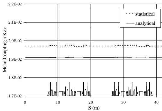
Figure 1 : Mean vertical coupling obtained by a complete analytical derivation along a half period.
