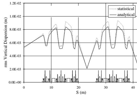
Figure 3 : One standard deviation of the resulting vertical spurious dispersion along a half period.
