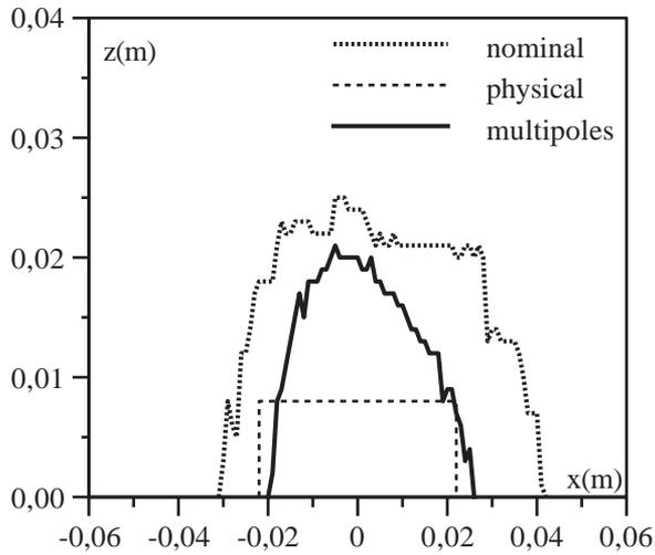
Fig. 2. Effect of multipolar components of sextupoles on dynamic aperture.
