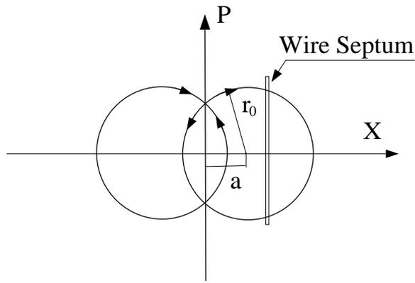
Figure 4: Extraction beam trajectory in phase space
