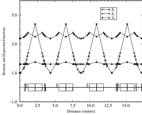
Figure 3: The CIS lattice functions  $\beta_x$ ,  $\beta_z$  and  $D_x$  for  $L = 2.0$  m,  $\theta_e = 12^\circ$
