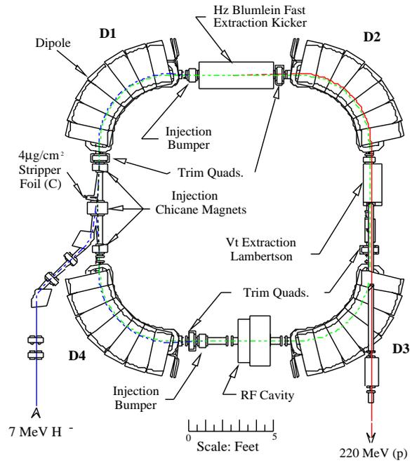
Figure 1: The general layout of the Indiana University Cyclotron Facility Cooler Injector Synchrotron at IUCF
