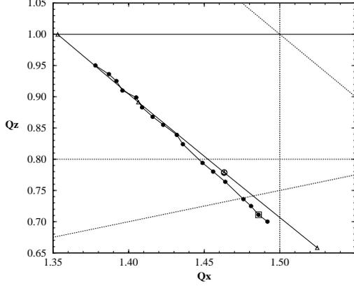
Figure 2: Tune shift by four symmetrical trim quads. Where  $\circ$  stand for CIS working point,  $\triangle$  for the calculation curve,  $\bullet$  for the experimental measurement, and  $\square$  for the tune with chicane dipoles but zero trim quad current.
