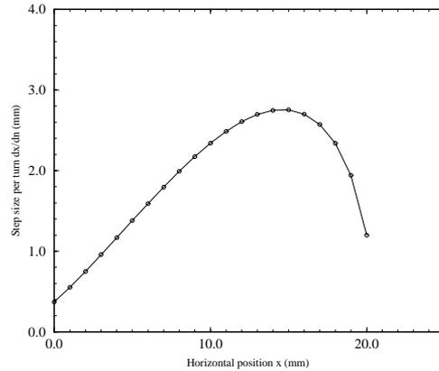
Figure 5: Step size of the extracted beam versus horizontal position. Wire septum is at  $x = 15$  mm.  $r_0 = 12$  mm,  $a = 8.5$  mm.
