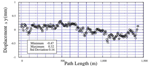
Fig. 3 Alignment results for vertical direction.
