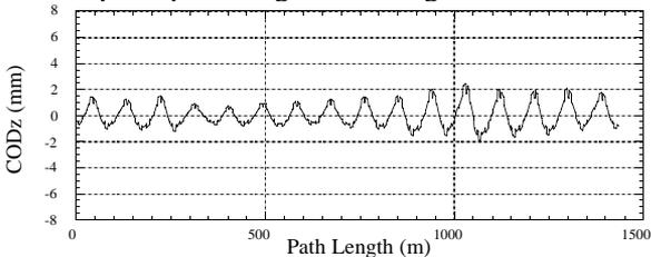
Fig. 7 Vertical closed orbit distortion resulting from random quadrupole magnet misalignment on a girder.
