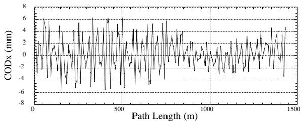
Fig. 6 Horizontal closed orbit distortion resulting from random quadrupole and girder misalignment.
