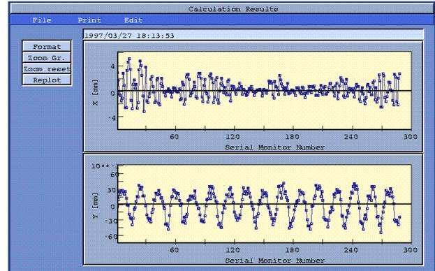
Fig. 10 Observed closed orbit distortion.
