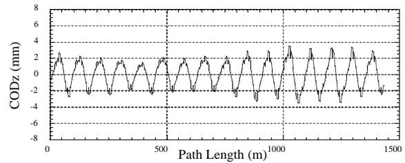
Fig. 9 Vertical closed orbit distortion resulting from random quadrupole and girder misalignment.
