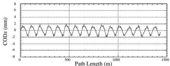
Fig. 8 Vertical closed orbit distortion resulting from girder misalignment.
