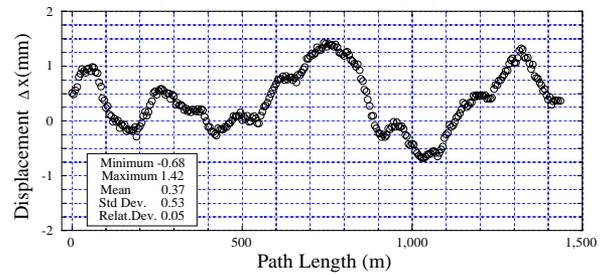
Fig. 2 Alignment results for horizontal direction.
