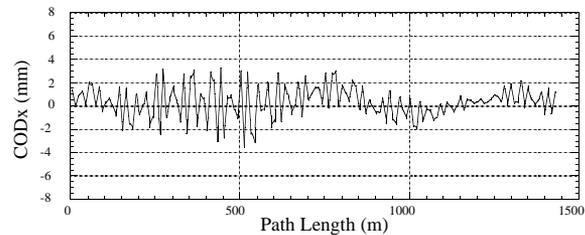
Fig. 5 Horizontal closed orbit distortion resulting from girder misalignment.
