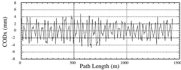
Fig. 4 Horizontal closed orbit distortion resulting from random quadrupole magnet misalignment on a girder.
