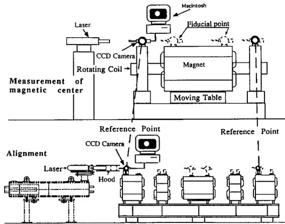
Fig. 1 Measurement of magnetic center and alignment of quadrupole and sextupole magnets on a girder.
