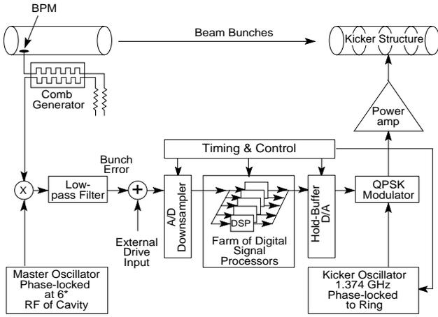
Figure 1: Feedback system (courtesy SLAC LFB group).
