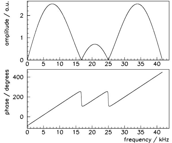
Figure 2: Frequency response of the 5-tap FIR filter.
