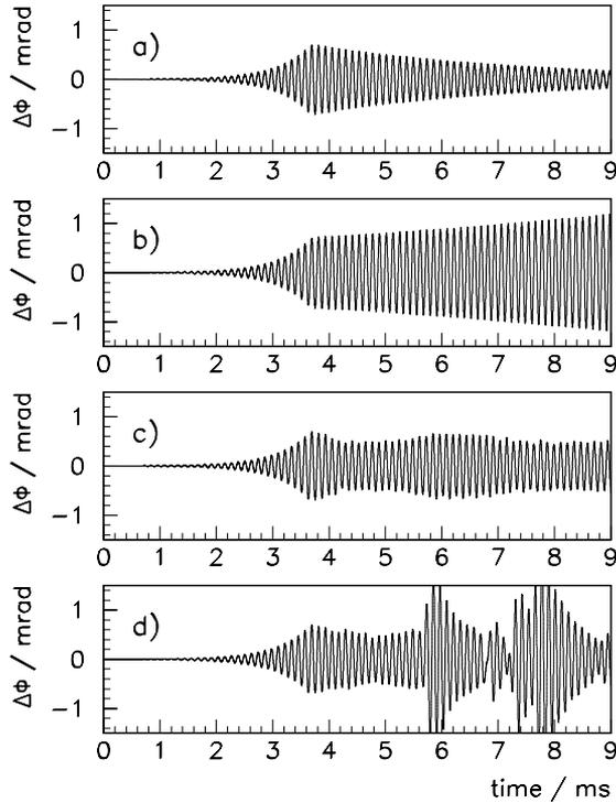
Figure 4: Phase oscillation driven by a cavity HOM and damped by the feedback system after  $t = 3.6$  ms (see text).
