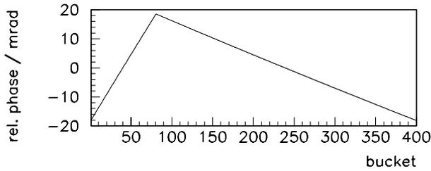
Figure 3: Relative synchronous phase with 20% bunch gap.
