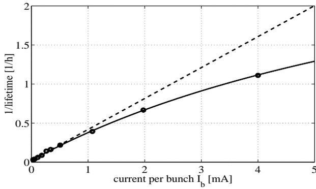
Figure 3: Inverse lifetime versus bunch current at 1.5 GeV. The total current was kept constant at 8 mA.
