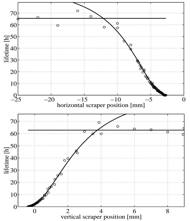
Figure 2: Lifetime as a function of the horizontal (upper) and vertical (lower) scraper position. The storage ring parameters were 5 mA in 288 bunches, beam energy 1.5 GeV.
