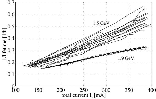
Figure 1: Inverse beam lifetime as a function of the total current for standard user operations. Each line represents a 4 hour user run. The upper curves show the lifetime for 1.5 GeV, while the lower curves are for 1.9 GeV operation.
