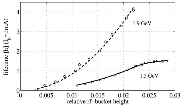
Figure 4: Lifetime versus rf-bucket height for 1.9 GeV (dashed line) and 1.5 GeV (solid line). 8 mA in 8 bunches were stored.
