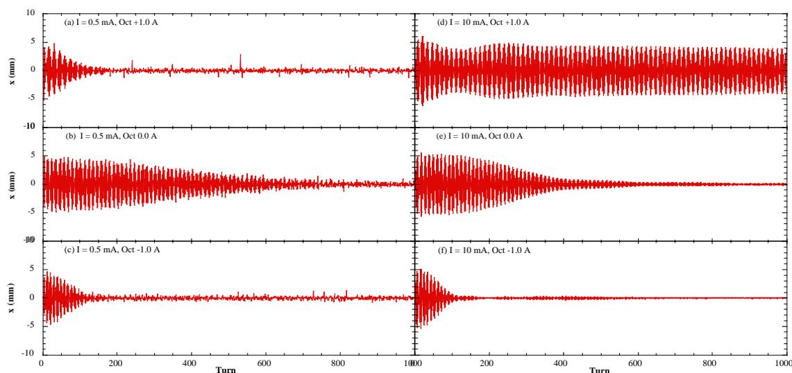
Figures 1: The horizontal beam centroid motions measured at a current of 0.5 mA and 10mA are shown as a function of turn. The left sides of the figure are for 0.5 mA and the right parts for 10 mA. The upper parts are for +1.0 A, the middle parts for 0.0 A, and the lower parts for -1.0 A.
