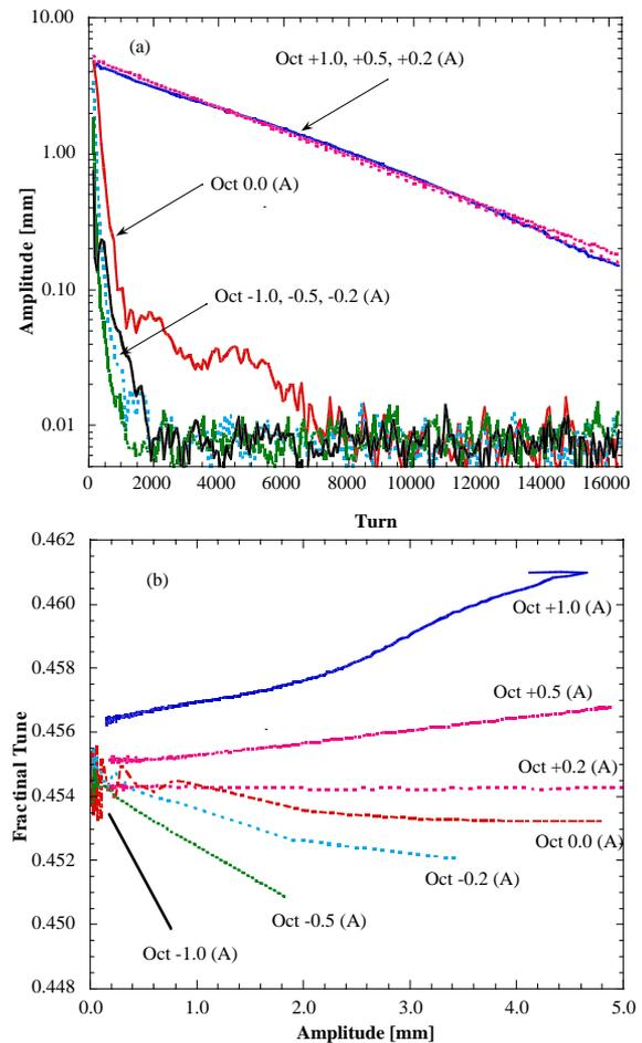
Figures 2: (a) Amplitudes of coherent centroid motions are derived by STFT method. (b) Amplitude dependent tune shift
