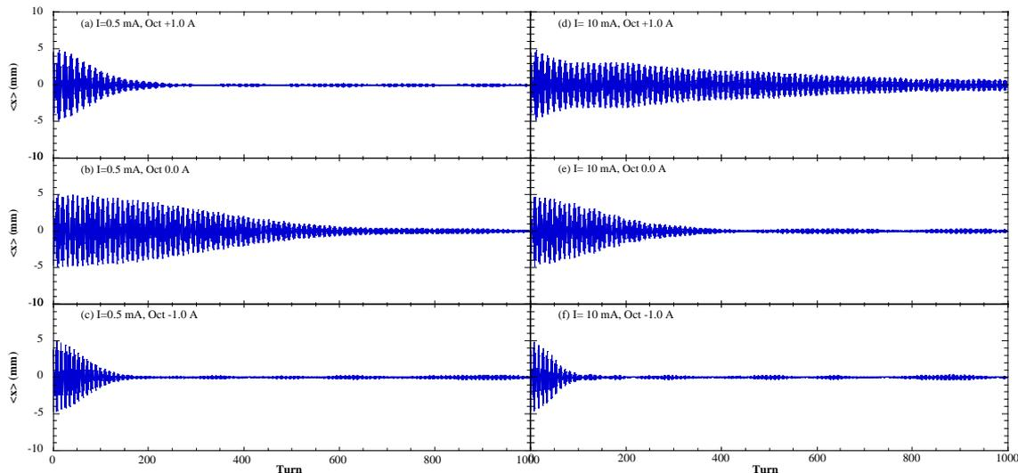
Figures 3: The expected horizontal beam centroid motions calculated at a current of 0.5 mA and 10mA by multi-particle tracking method are shown as a function of turn. The left sides of the figure are for 0.5 mA and the right parts for 10 mA. The upper parts are for +1.0 A, the middle for 0.0 A, and the lower for -1.0 A.
