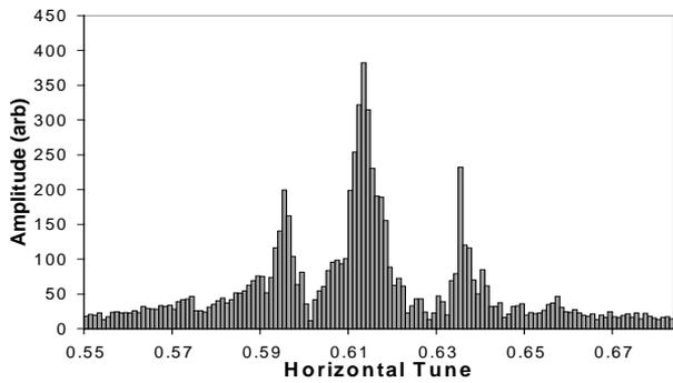
Figure 3.2a: Measured horizontal spectrum of the betatron motion of positrons in SPS
