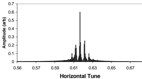
Figure 3.2b: Simulated horizontal betatron spectrum for a comparable chromaticity as in fig 3.2a
