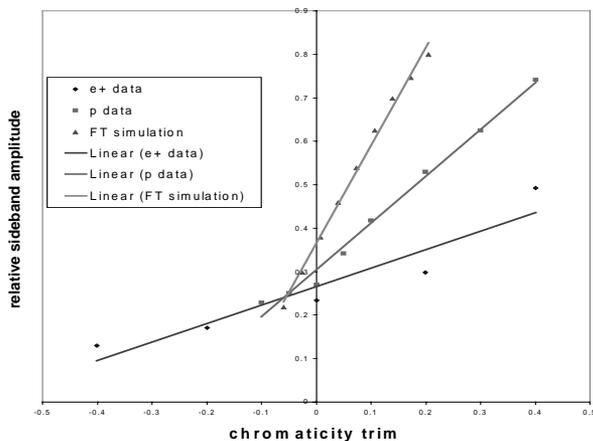
Figure 3.2c relative amplitude of synchrotron sidebands as function of chromaticity trim.
