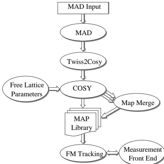
Figure 1: Flow chart of the FM tracking tools
