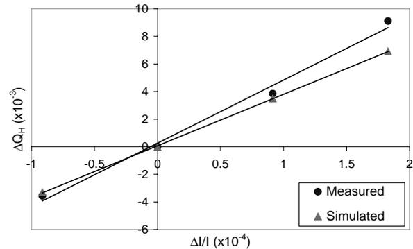
Figure 3.1: Horizontal tune as a function of change in current in the main QD quadrupole string
