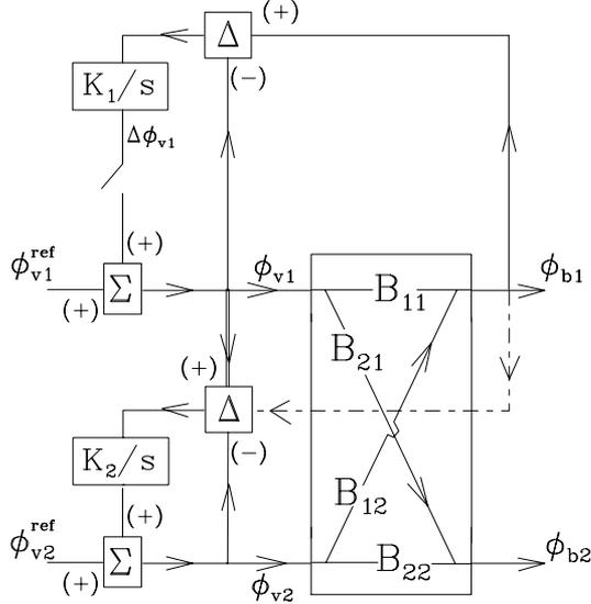
Figure 4: system schematic for 2nd harmonic locked to voltage (bold line) or beam (dashed) fundamental
