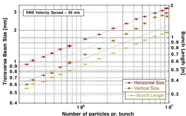
Figure 5: The transverse and longitudinal dimensions of the laser-cooled beam as a function of the current. The colored lines are cuberoot fit to the data, whereas the black line is a parallel translation of a cuberoot fit to guide the eye. The beta functions at the point of measurement are  $\beta_x = 12.1\text{m}$  and  $\beta_y = 2.6\text{m}$ .
