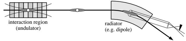
Figure 1: Principle of the generation of short x-ray pulses.
