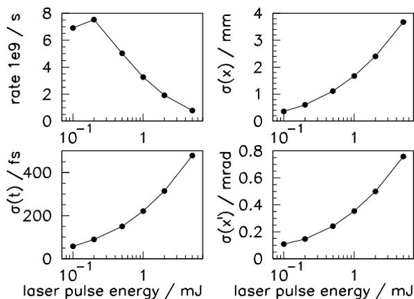
Figure 4: Electron rate and rms width in  $x$ ,  $x'$  and time.
