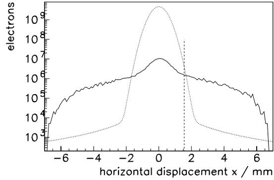
Figure 3: Horizontal beam profile (dotted) and distribution of energy-modulated electrons (solid line) in the U-55.
