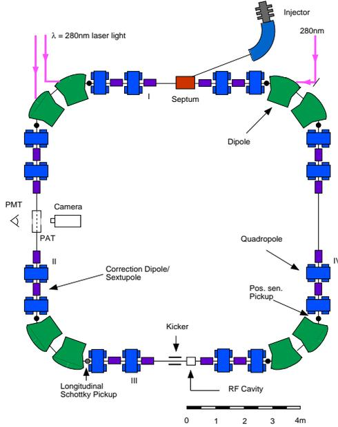
Figure 2: The ASTRID Storage Ring. One of the cooling lasers is split to provide light for the probe section (II) in which both the velocity profiles, and the transverse spatial profiles are measured.
