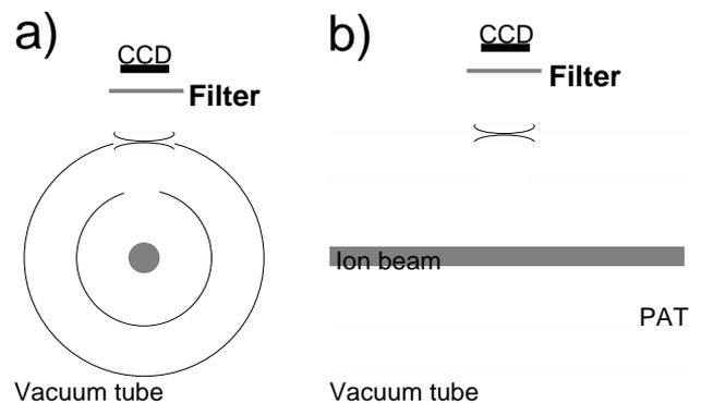
Figure 1: Schematic drawing of the experimental arrangement for imaging the horizontal beam size. a) Downstream view, b) Side view. The filter is a UV filter to block out most of the light coming from other sources than the beam.
