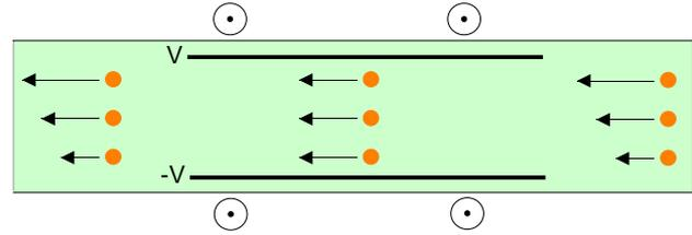
Figure 5: Tapered cooling by introducing a horizontally varying potential by exciting two parallel plates around the beam. The magnetic field compensates for the bending that the electric field would otherwise cause.
