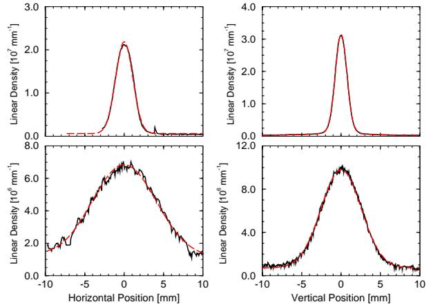
Figure 3: Horizontal and vertical particle distributions for uncooled (bottom) and cooled (top) beams of  $\sim 5.8 \cdot 10^7$  particles. The distributions have been normalized to have an area of  $5.8 \cdot 10^7$ . The dashed lines are gaussian fits to the distributions.
