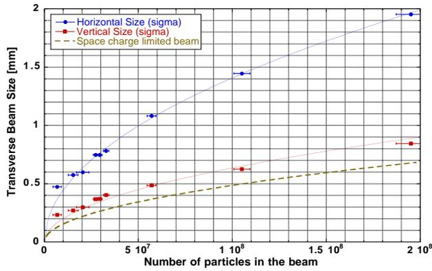
Figure 4: Transverse beam dimensions for a laser-cooled ion beam, as a function of the number of particles in the beam. The betafunions at the camera position where  $\beta_x=12.13\text{m}$  and  $\beta_y=2.61\text{m}$ . The solid curves are fits to the data, assuming the beam size varies as the squareroot of the number of ions. The dashed curve is the size of a space-charge limited beam for a betatron tune of  $Q_{\perp} = 2.5$ .
