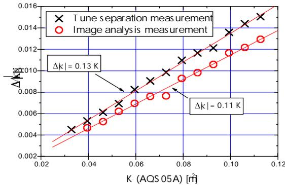
Figure 2: Measurement of the variation of  $|\kappa|$  as a function of quadrupole magnet strength in the low beta optics. Only skew quadrupole A is powered.
