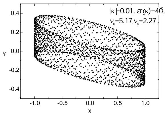
Figure 1: Example of integrated beam transverse profile which results from the calculated transverse map.
