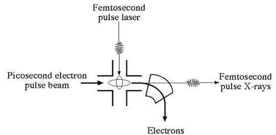
Figure 1: A schematic illustration of the fs X-ray generation by the inverse Compton scattering between a low emittance  $e^-$  beam and an intense fs laser light.
