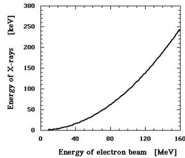
Figure 3: Energy of the X-ray photons vs energy of  $e^-$  beam.
