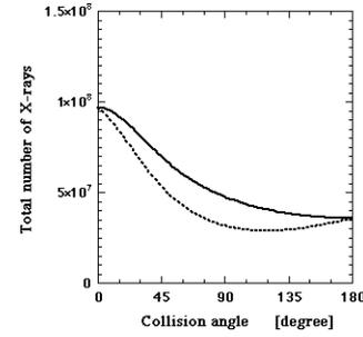
Figure 2: Total number of X-ray photons produced by linearly polarized lasers under the different interaction angles. The solid (dashed) line represents the polarization direction is parallel (perpendicular) to the scattering plane.
