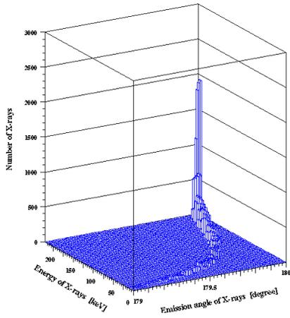
Figure 5: Energy and angular distributions of the X-rays produced under the linear inverse Compton scattering.
