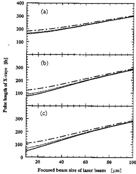
Figure 4: Pulse length of the X-rays produced by 10 (solid line), 50 (dashed line) and 100 fs (solid-dashed line) pulse laser. The  $e^-$  beams with the focused beam size of 50 (a), 20 (b) and 10  $\mu\text{m}$  (c) are used in the calculation.
