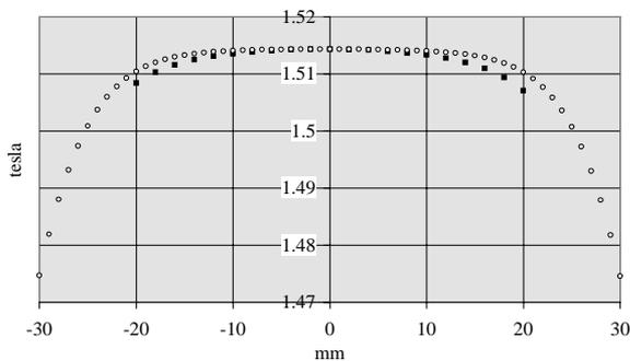
Figure 4: Transverse dipole field for high excitation.
