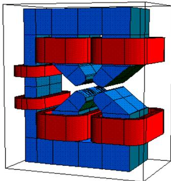
Figure 5: Quadrupole magnet.
