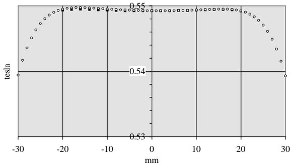
Figure 3: Transverse dipole field for low excitation.
