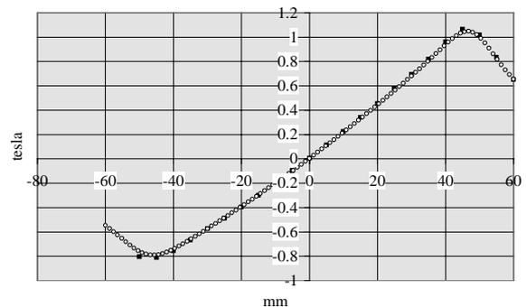
Figure 8: Transverse quadrupole field at high excitation.
