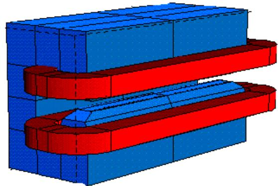
Figure 1: Dipole magnet.
