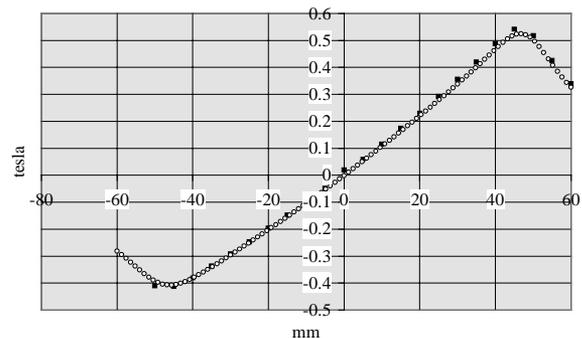
Figure 7: Transverse quadrupole field at low excitation.
