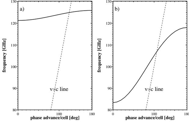
Figure 2: Dispersion diagram of the first a) accelerating and b) deflecting mode of a 120 GHz,  $2\pi/3$ -mode structure.
