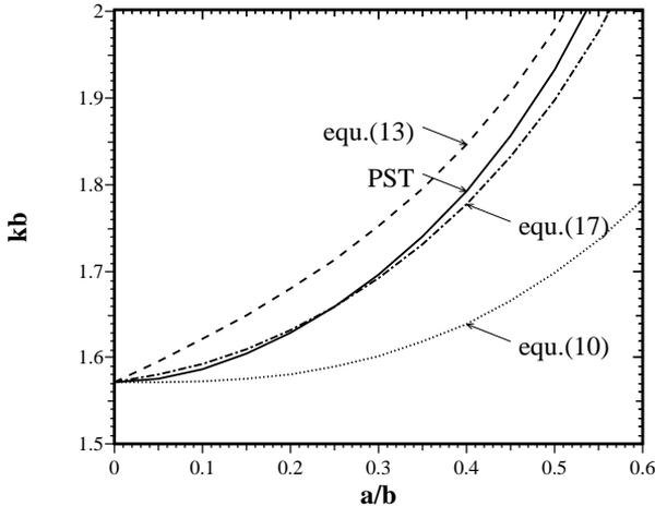
Figure 4: Normalized frequency versus  $a/b$  for the accelerating mode with  $M = 0$  and  $v_{ph} = c_0$ .
