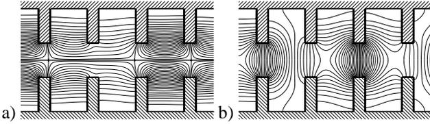
Figure 3: Lines  $H_x = \text{const.}$  of the first a) accelerating and b) deflecting mode of a 120 GHz,  $2\pi/3$ -mode structure ( $v_{ph} = c_0$ ).
