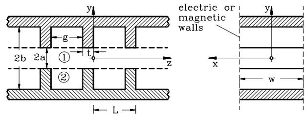
Figure 1: Longitudinal and transverse cross-sections of a rectangular structure.
