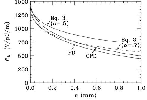
Figure 2: The wakefield of our periodic model, as obtained by different frequency domain methods.
