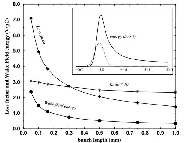
Figure 1: Loss factor and the wake field energy, following the bunch in the tube, after a single cell of the TESLA cavity over the bunch length. Ratio of field energy to the loss factor is multiplied by 10 (to use the same scale).
