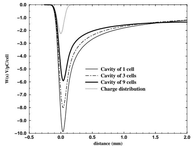
Figure 7: Wakes of a 50  $\mu$  bunch in cavities with a different number of cells
