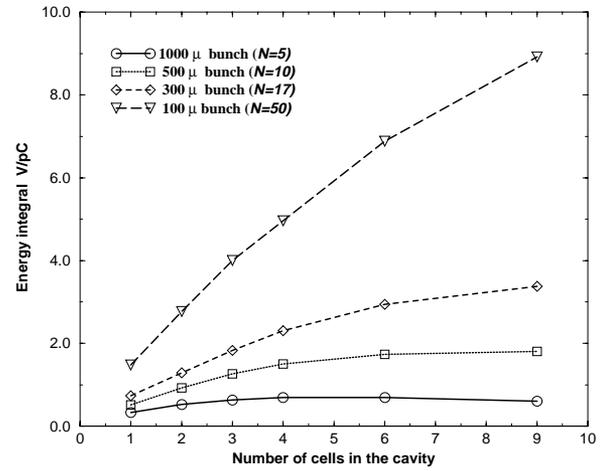
Figure 4: Wake field energy, following the bunch in the TESLA cavity, for bunchlength of 1 mm, 0.5 mm and 0.1 mm.
