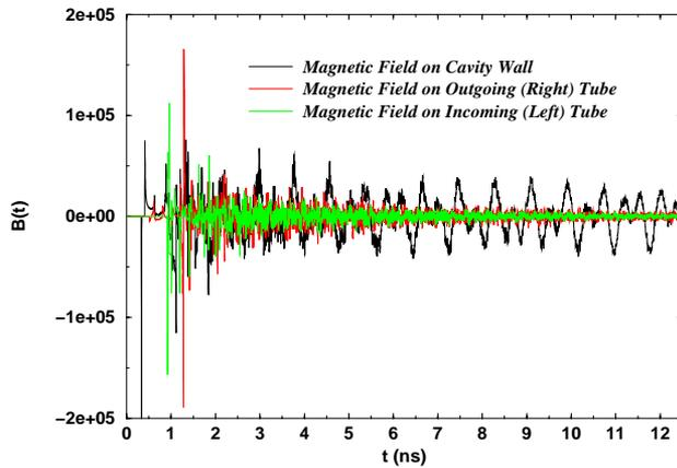
Figure 2: Magnetic field, monitored on different position on the cavity and tube surface
