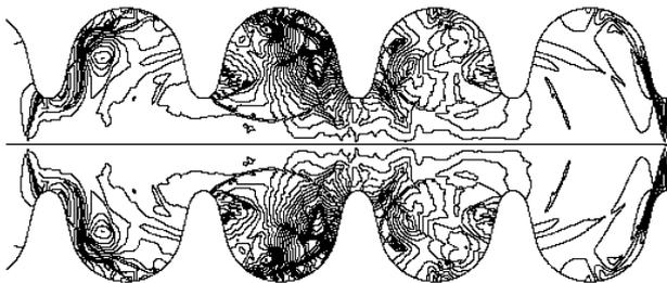
Figure 6: Electric force lines in TESLA cavity, after "excitation" of one cell
