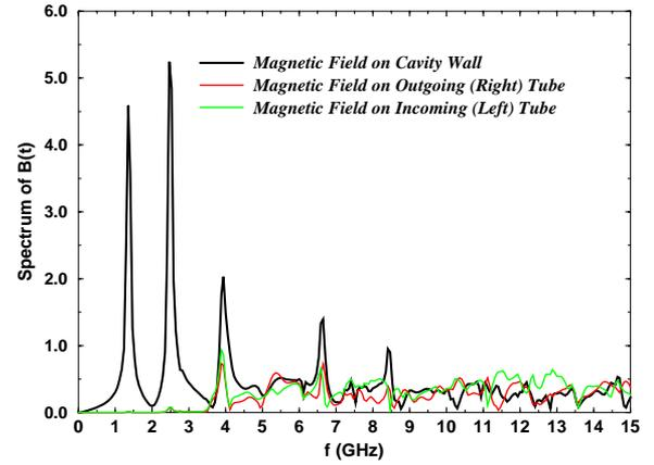
Figure 3: Amplitudes of Fourier transform of magnetic field, monitored on different position on the cavity and tube surface
