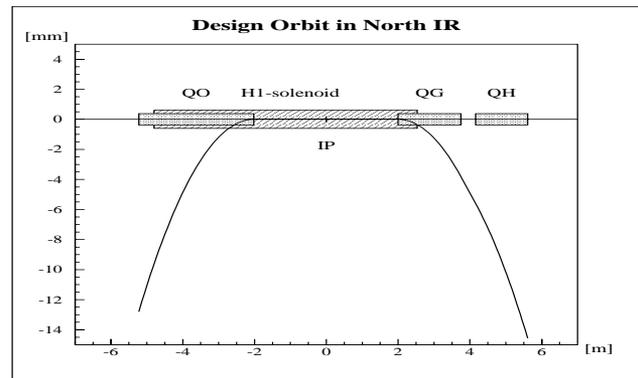
Figure 1: The curved design orbit inside H1 solenoid
