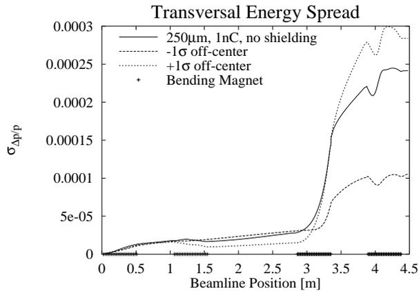
Figure 3: Induced transversal rms energy spreads for different longitudinal positions
