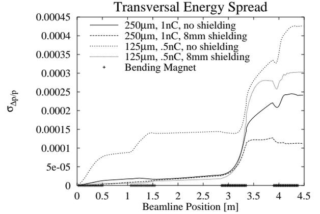
Figure 1: Induced transversal rms energy spreads for different parameter sets
