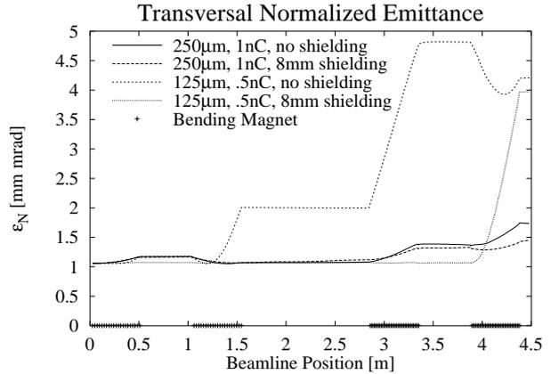
Figure 2: Normalized transversal statistical slice emittance for different parameter sets
