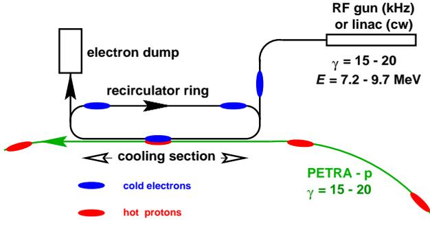
Figure 1: Basic idea of electron cooling by bunched electron beam. The electron bunches match in space the hadron bunches, hence the virtual electron beam power is substantially reduced. Further power reduction might be achieved using recirculator
