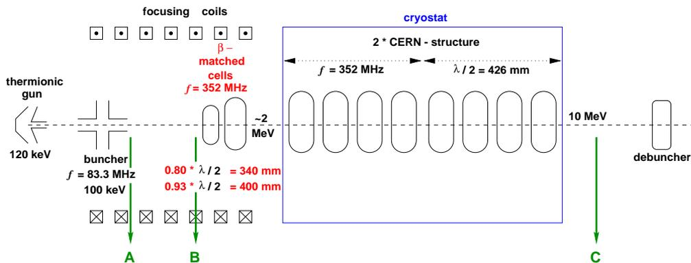
Figure 2: Basic design scheme of the injector linac
