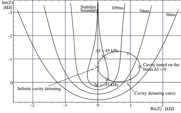
Figure 1: Stability diagram, rise time trajectories and cavity detuning curve ( $\Delta f$  spanning from  $-\infty$  to  $+\infty$ ).
