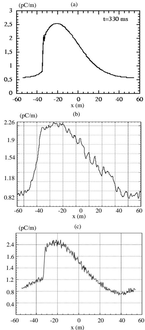
Figure 4: Distribution of the line charge density during the wave steepening phase: (a) cold fluid model; (b) ESR measurements; (c) PATRIC simulation.
