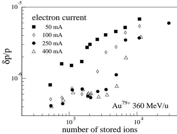
Figure 3: Momentum spread of a  $\text{Au}^{79+}$  beam at 360 MeV/u cooled by different electron currents.
