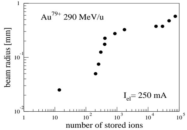
Figure 2: Beam radius determined from the scraper position as a function of the number of  $\text{Au}^{79+}$  ions (energy 290 MeV/u) which remained stored in the ring (cooled with an electron current of 250 mA,  $n_e = 4.1 \times 10^6 \text{ cm}^{-3}$ ).
