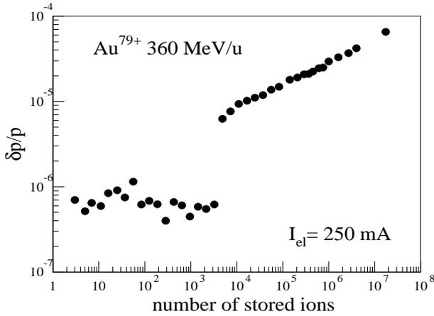
Figure 1: Momentum spread versus number of stored ions for a  $\text{Au}^{79+}$  beam at 360 MeV/u which was cooled with an electron current of 250 mA ( $n_e = 3.8 \times 10^6 \text{ cm}^{-3}$ ).
