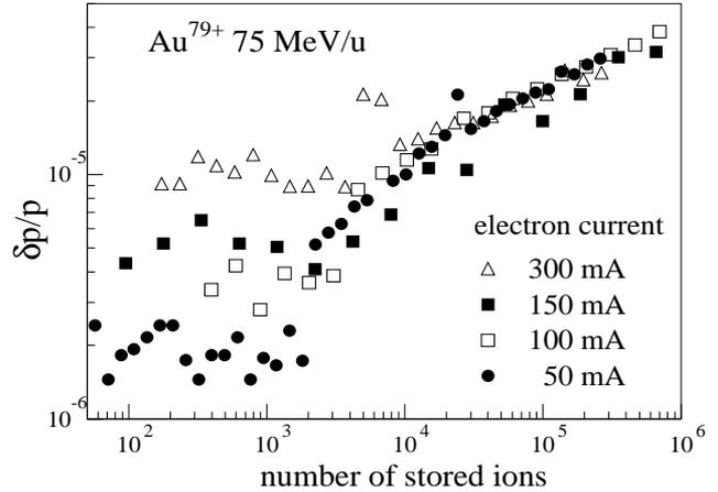
Figure 4: Momentum spread of a  $\text{Au}^{79+}$  beam at 75 MeV/u cooled by different electron currents.
