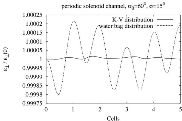
Figure 1: Transverse emittance functions within a periodic solenoid channel for K-V and “water bag” phase space density profiles with  $\sigma_0 = 60^\circ$  and  $\sigma = 15^\circ$ .
