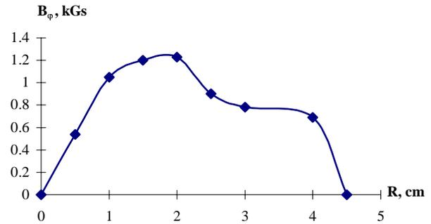
Figure 1: The distribution of azimuthal magnetic field  $B_\phi$  on radius ( $U_n = 6$  kV,  $l = 4$  cm).
