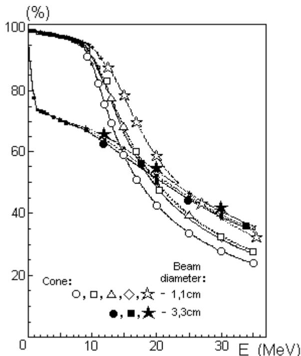
Figure 8: Energy collection coefficient for FC-REB transducer
