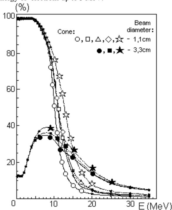
Figure 7: Charge collection coefficient for FC-REB transducer
