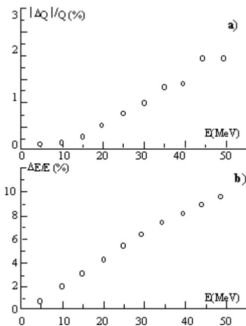
Figure 5: Charge and energy leakage for FC-1 transducer
