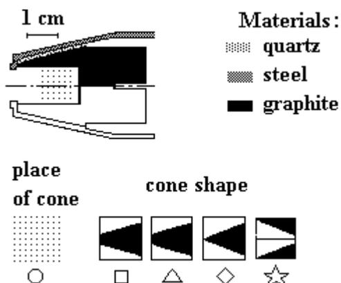
Figure 6: Sketch of the FC-REB transducer
