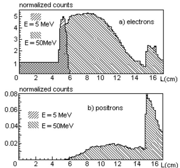
Figure 2: Allocation of electron and positron flow along the absorber
