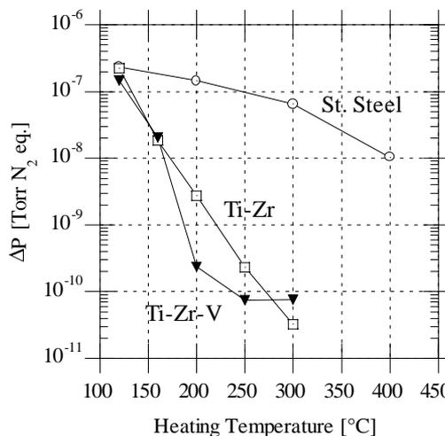
**Fig. 3:** Comparison of ESD measurements for stainless steel, TiZr and TiZrV coatings. Experimental conditions as described for Fig. 1.
