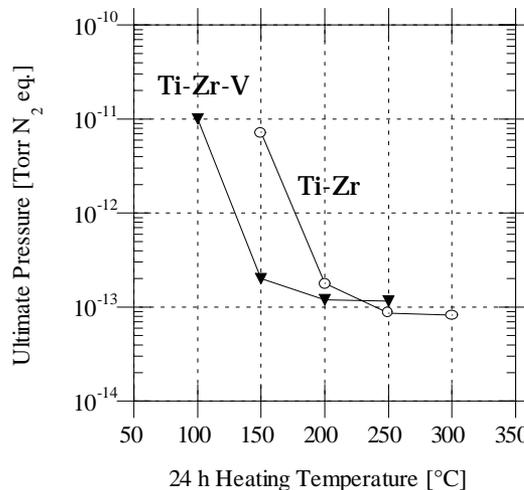
**Fig. 4:** Ultimate pressures obtained after 24 h baking cycles, without intermediate air venting, on chambers coated with TiZr and TiZrV. Chamber length 2 m, diameter 10 cm, applied pumping speed  $25 \lambda s^{-1}$  for  $H_2$ .
