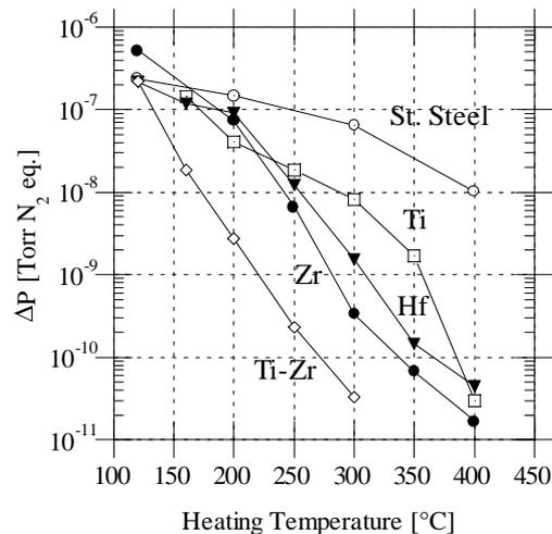
**Fig. 1:** Total pressure increase induced by electron bombardment of stainless steel, uncoated or coated with Ti, Zr, Hf, and equiatomic TiZr.
