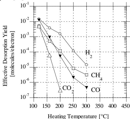
**Fig. 2:** Effective desorption yield of  $H_2$ ,  $CH_4$ ,  $CO$ ,  $CO_2$  for an equiatomic TiZr coating. Experimental conditions as described for Fig. 1.
