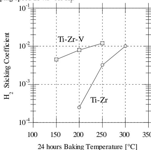
**Fig. 5:** Variation of the  $H_2$  sticking coefficient for TiZr and TiZrV coated chambers as a function of baking (24 h) temperature. Data obtained by gas injection and Monte Carlo simulation.
