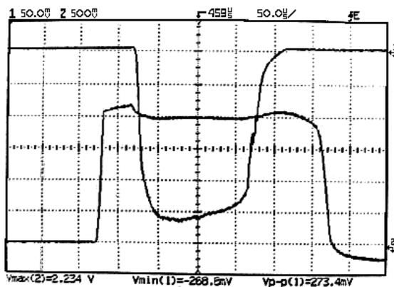
Figure 4: H<sup>-</sup> beam current (negative pulse) and 4.0 kV extraction voltage, 50 ns/div.
