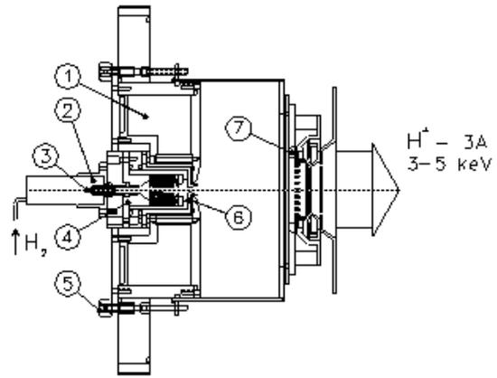
Figure 2: The BINP-type proton source: (1) solenoid; (2) pulsed valve; (3) trigger electrode; (4) cathode; (5) alignment screw; (6) anode; (7) proton extraction grids.
