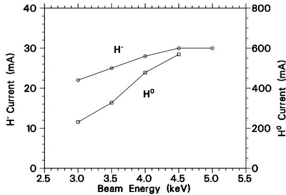
Figure 3: H<sup>-</sup> ion current and H<sup>0</sup> beam intensity within the Na negative-ionizer acceptance versus beam energy.
