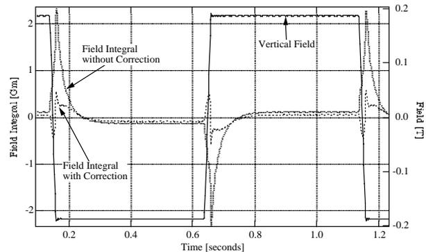
Figure 7 : Vertical field and field integrals as function of time for a 1 Hz repetition rate. The current is flipped between -250 A and 250 A within 20ms. The magnetic gap is 16 mm.
