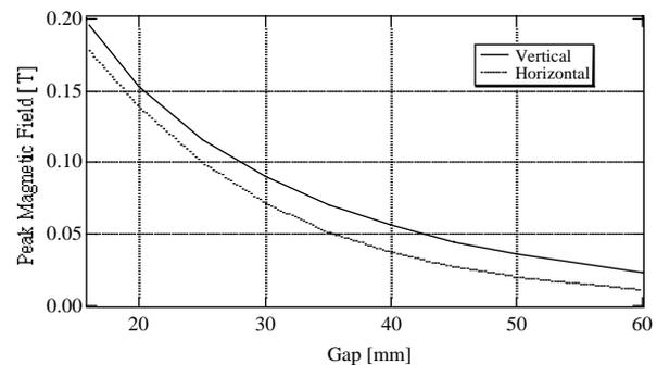
Figure 4 :Peak horizontal and vertical fields as a function of the magnetic gap for a current of 250 A.
