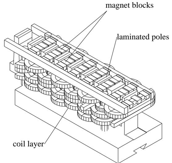
Figure 1: 3D view of the termination of the undulator.
