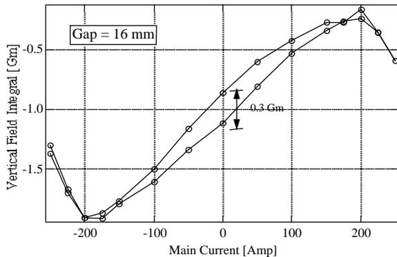
Figure 5 Hysteresis cycle of field integral vs. Current in the coil for a magnetic gap of 16 mm.
