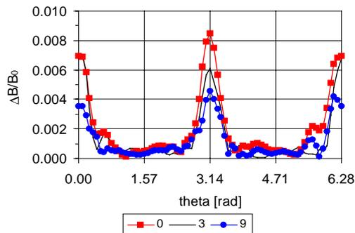
Figure 4: Relative field error at the walls of the vacuum chamber for sextupole SH at 200 A
