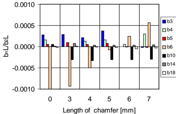
Figure 1: Relative multipole components of Q390 at 300 A using chamfers of different lengths. The normal components are shown
