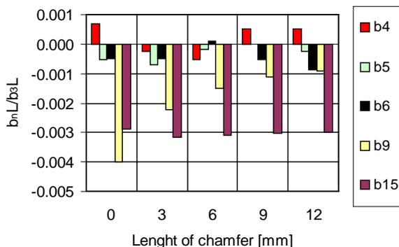
Figure 3: Relative multipole components of SH at 200 A using chamfers of different lengths. Normal components
