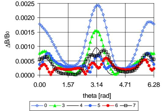
Figure 2: Deviation from the pure quadrupolar field at the walls of the vacuum chamber for quadrupole Q390 with different chamfers at 300 A
