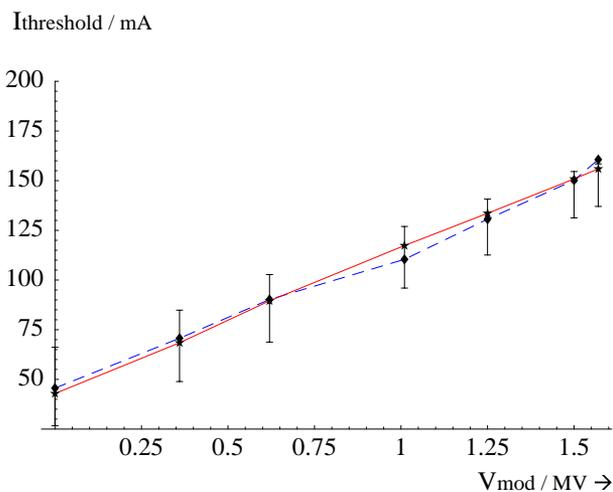
Figure 1: Threshold current for homogenous filling, applying voltage modulation with cavities 5 & 6 operated at  $f_{RF} + f_0$  for Landau damping [6]
