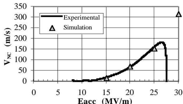
Figure 8: Experimental and simulated normal zone propagation velocity as a function of the accelerating field.
