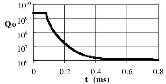
Figure 6: Quality factor decay during the cavity quench.
