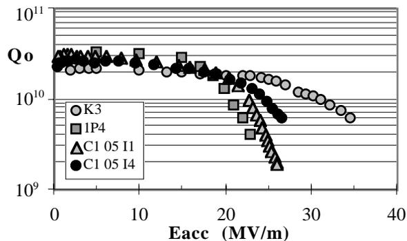
Figure 1:  $Q_0$  degradation at high field without X-rays or electrons for different cavities: K3 (KEK), 1P4 (LNL spun cavity), C1-05 I1 and C1-05 I4 (Saclay).
