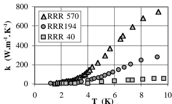
Figure 9: Thermal conductivity for numerical simulations.
