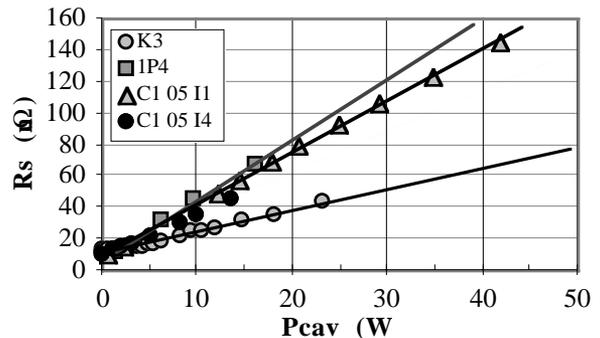
Figure 2: Variation of the surface resistance with the dissipated power in several cavities.
