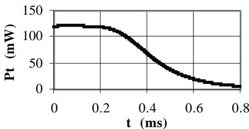
Figure 5: Transmitted power recorded during a quench in a 1.3 Ghz single-cell cavity (test C1-05 I1).
