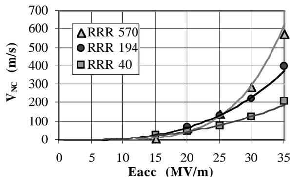
Figure 10: Calculated normal zone expansion velocity as a function of  $E_{acc}$  for different RRR ( $R_S^N = 2 m\Omega$ ).
