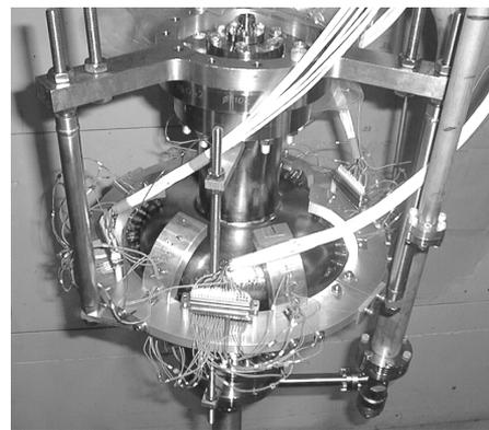
Figure 3: Thermometric apparatus mounted on the cavity.
