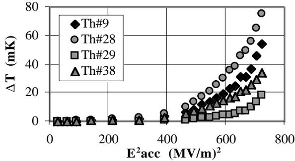
Figure 4: Heating measured on cavity C1-10 vs  $E_{acc}^2$ .
