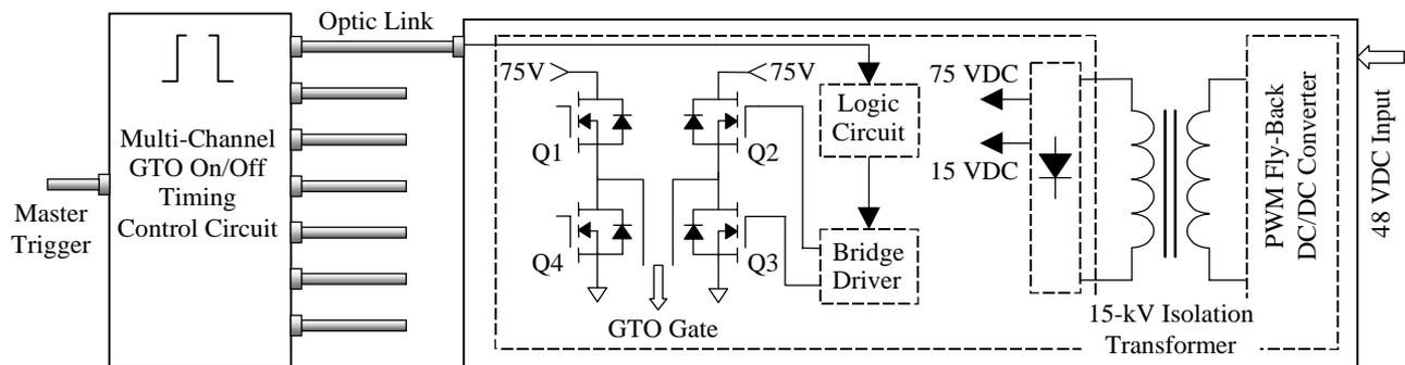
Figure 7. Block diagram of the GTO gate drive.
