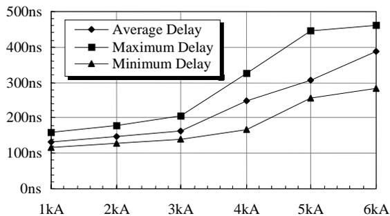
Figure 4. GTO turn-on delay versus peak current.
