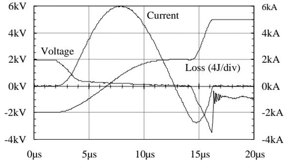
Figure 3. GTO voltage, current, and switching losses.
