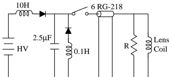
Figure 1. Circuit diagram of the pulser.
