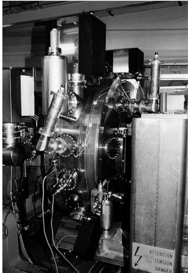
Figure 4: 80 MHz cavity after installation in the PS tunnel.
