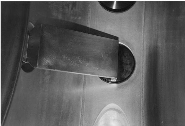
Figure 3: Power coupling loop mounted inside the cavity.
