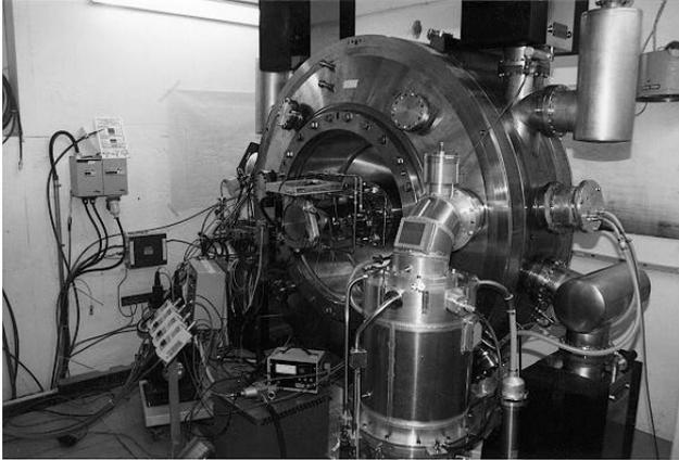
Figure 2: Cavity and amplifier in the test stand.
