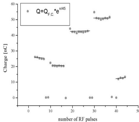
Figure 3: Corrected plot of dark current vs. number of RF pulses.
