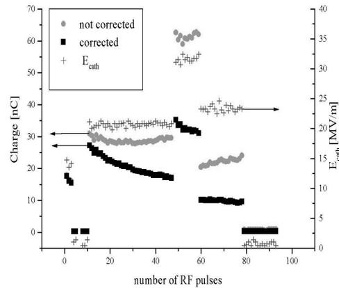
Figure 5: Dependence of charge in Faraday cup and quantum efficiency upon number of RF pulses.
