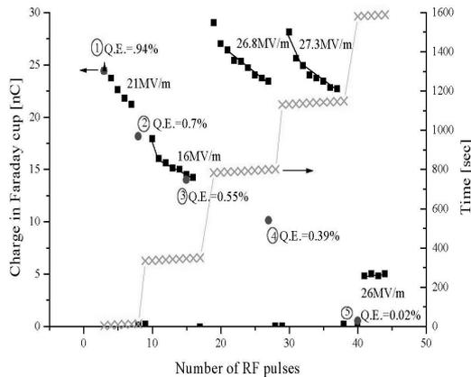
Figure 2: Dependence of charge in Faraday cup and quantum efficiency upon number of RF pulses.
