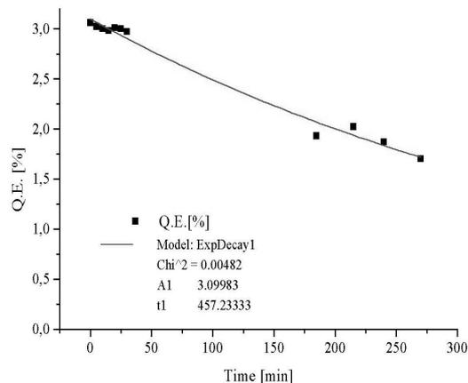
Figure1: The dependence of quantum efficiency of GaAs photocathode upon time measured in activation chamber.
