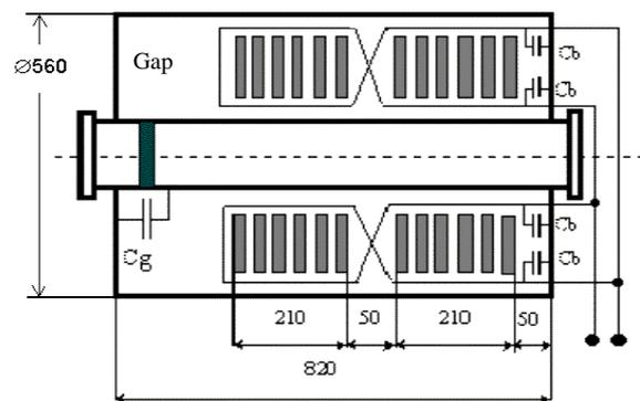
Figure 4: Schematic drawing of the RF cavity.
