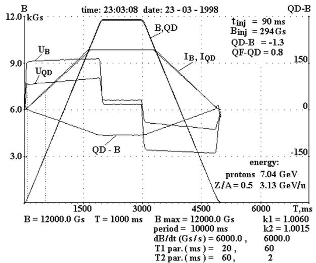
Figure 3: Example of magnetic field cycle parameters.
