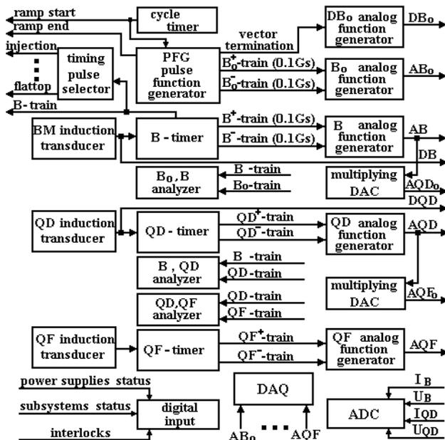
Figure 2: Schematic diagram of the MPSC.
