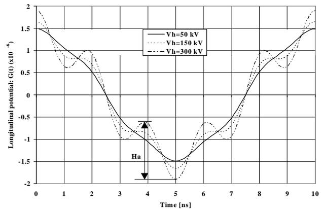
Figure 1: Longitudinal potential for 3 harmonic voltages
