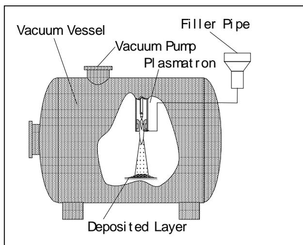
Figure 1: Schematic view of the vacuum-plasma-spraying (VPS) equipment for fabricating thin films of metal alloys or of carbon nanotubes.
