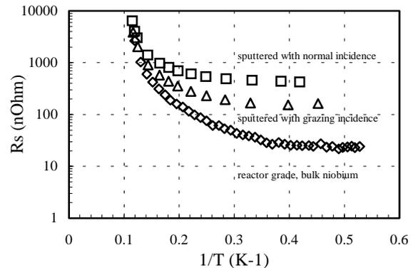
Figure 7 :  $R_s$  versus  $1/T$  for the 3 samples.
