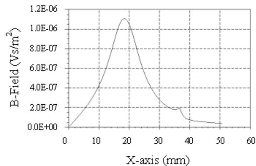
Figure 3 : Magnitude of the surface field on a line from the disk center to its edge passing in between the two half loops
