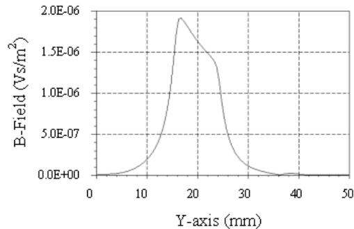
Figure 2 : Magnitude of the surface field on a line from the disk center to its edge passing under the center of a half loop
