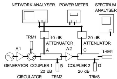
Figure 2. Measurement block diagram.
