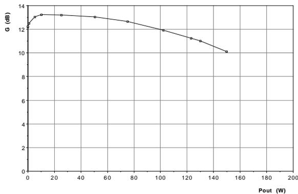
Figure 3. Gain versus output power.
