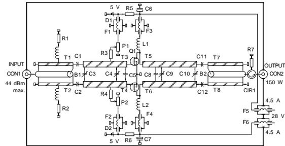
Figure 1. Schematic diagram of 150 W module.
