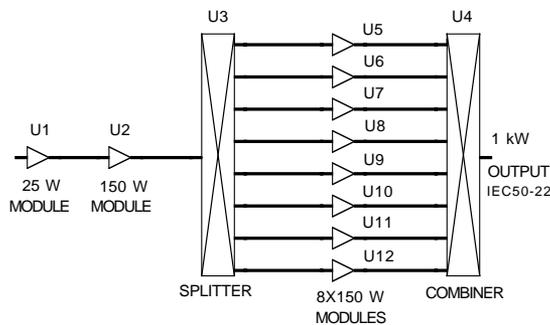
Figure 6. 1 kW amplifier block diagram.
