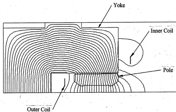
Figure 3: Computed magnetic flux line.
