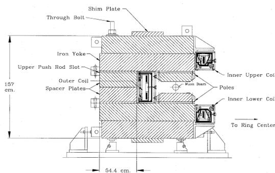
Figure 1: Magnet cross section
