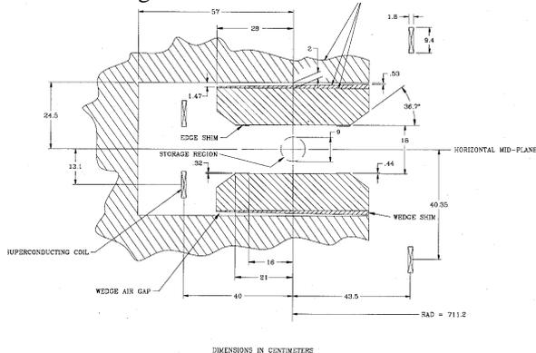
Figure 2: Cross section view of magnet gap region
