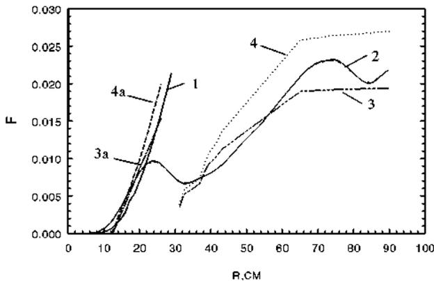
Figure 5: Flutter in dependence on cyclotron radius: 1 — the data of the measurements on model with straight sectors  $k_1 = 1.33$  (central part); 2 — the data of measurements on model with  $k_2 = 8$ ; 3 — calculations on the base of proposed methodology with  $2g_V = 284$  mm and the sector height  $h_1 = 69$  mm; 4 — calculations with  $2g_V = 386$  mm,  $h_1 = 108$  mm; 3a, 4a — calculations with straight sectors accordingly  $2g_V$  and  $h_1$ .
