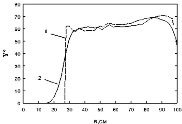
Figure 6: Spiral angle in dependence on cyclotron radius: 1 — geometry data of  $k_2 = 8$  model; 2 — experimental values.
