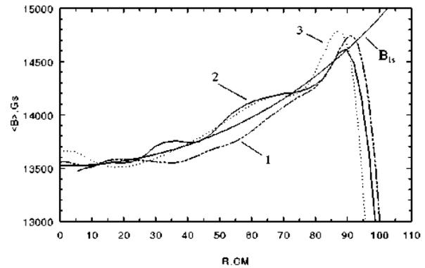
Figure 2: Average fields received for the scale models with  $k_1 = 1.33$  (1) and  $k_2 = 8$  (2);  $B_{is}$  – isochronous field; (3) – POISSON calculation results.
