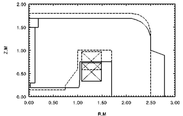
Figure 1: The reconstruction magnet SP-72 into magnet isochronous cyclotron. Dotted line is a contour of the initial magnet and solid line is a result of the reconstruction.
