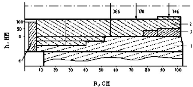
Figure 3: Shim profile in the hill and valley: 1–pole tip, 2–sector, 3–valley’s shim, 4–central plug.
