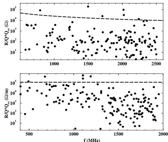
Fig. 6 : Damping of longitudinal (top) and dipole (bottom) HOMs by tapers and L- and D-couplers.
