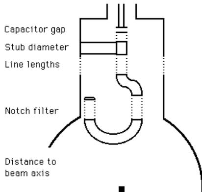
Fig. 2 : Sketch of the variable elements of D-coupler
