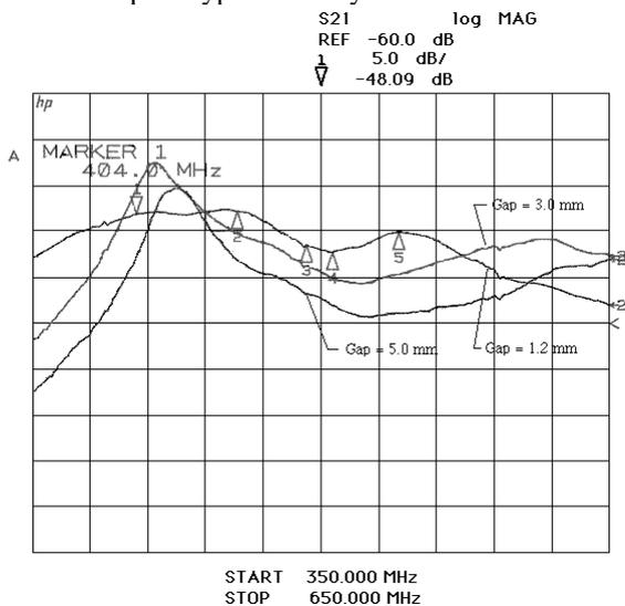
Fig. 3 : Transfer function of the D-coupler for various capacitor gaps.
