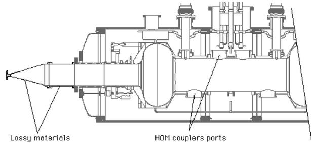
Fig. 1 : Layout of the cryostat with cavities and HOM dampers.
