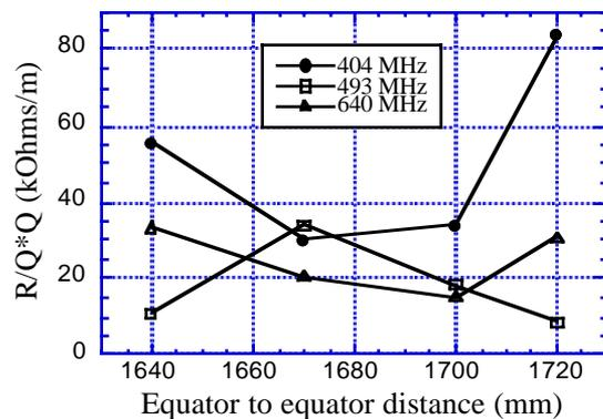
Fig. 5 : Dampings of the most dangerous dipole modes for different inner tube length.
