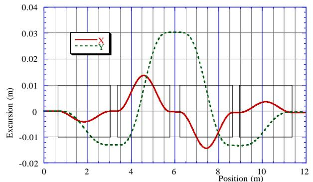
Fig. 6: Beam Orbit in a Siberian Snake.
