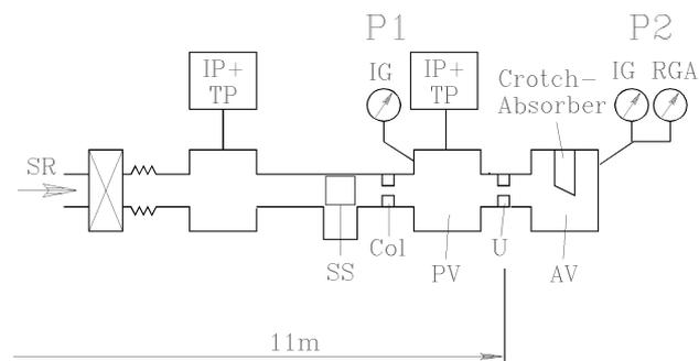
Figure A. Experimental installation for photodesorption test.
