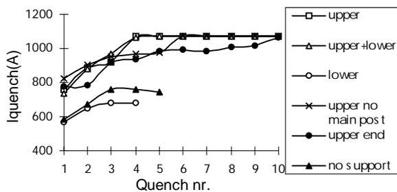
Figure 5: Training in free condition. Different coil supports.
