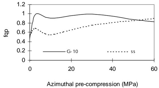
Figure 3: Evolution of the quality factor with the pre-compression
