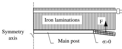
Figure 4: The bending effect in the coil end
